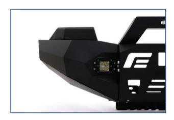
Our product is not an add-on to your existing bumper—it replaces it entirely. To install the Dakar steel front bumper, the original bumper must be removed.
